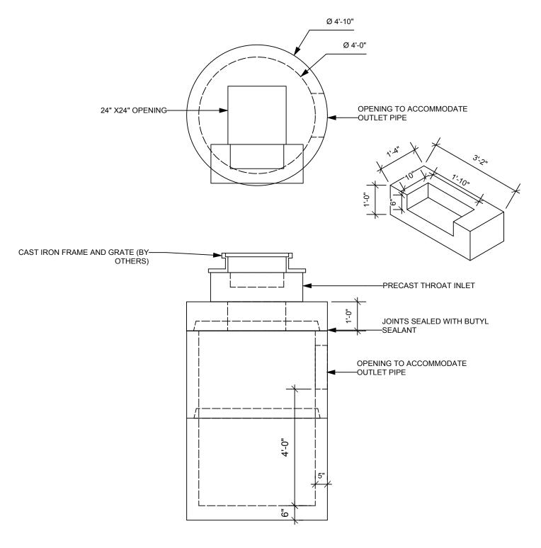
5000 PSI CONCRETE @ 28 DAYS MANUFACTURED TO MEET OR EXCEED ASTM SPEC C-478. H20 LOADING OPENINGS CAST AT REQUIRED LOCATIONS
